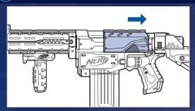
1. Pull SLIDE all the way back until READY INDICATOR is orange; keep in the rearmost position.
