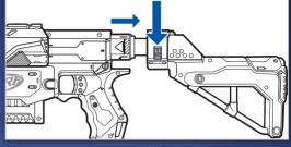
1. To remove STOCK, slide STOCK RELEASE SWITCH down.
